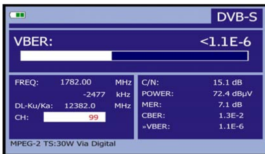
Figure 36.- DVB-S (QPSK) signals VBER measurement screen.
