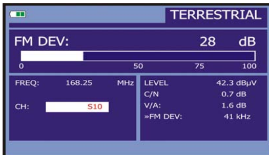
Figure 24.- FM carrier peak deviation.
