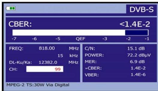
Figure 34.- DVB-S (QPSK) signals CBER measurement screen.
