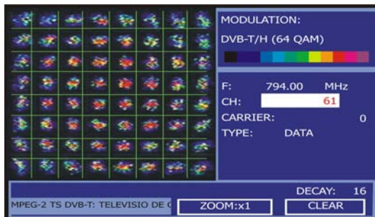
Figure 41.- Constellation Diagram. DVB-T/H (64 QAM) signal.
