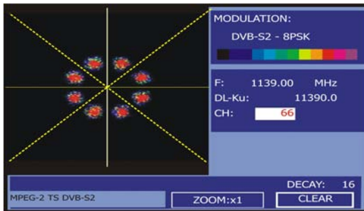
Figure 45.- Constellation Diagram. DVB-S2 (8PSK) signal.
