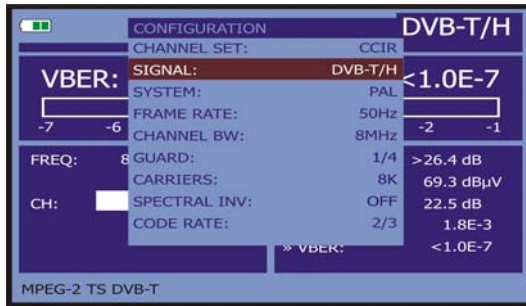
Figure 20.- Screen of measurement configuration (COFDM signals).
