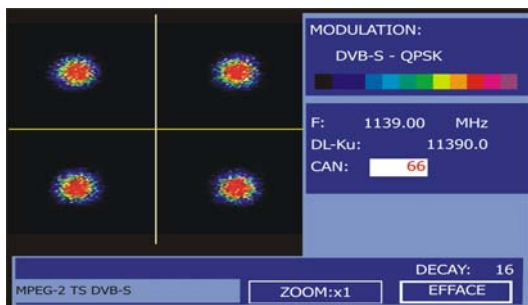
Figure 44.- Diagramme de constellation. Signal DVB-S (QPSK).
